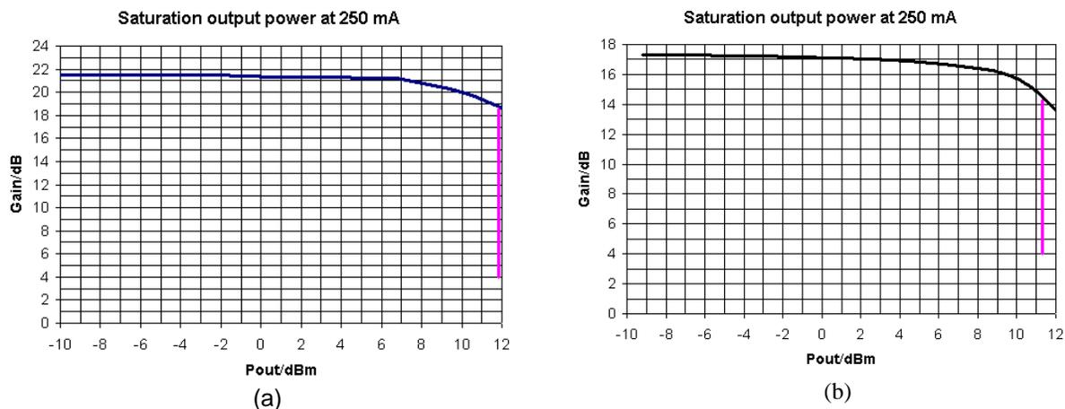
Fig. 2 Typical saturation output power as shown by the magenta line at 250 mA for:
