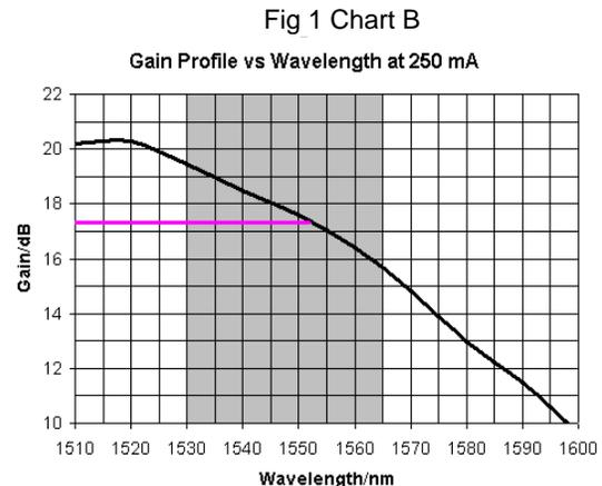
Figure 1 charts the typical gain profile versus wavelength at 250 mA for:
