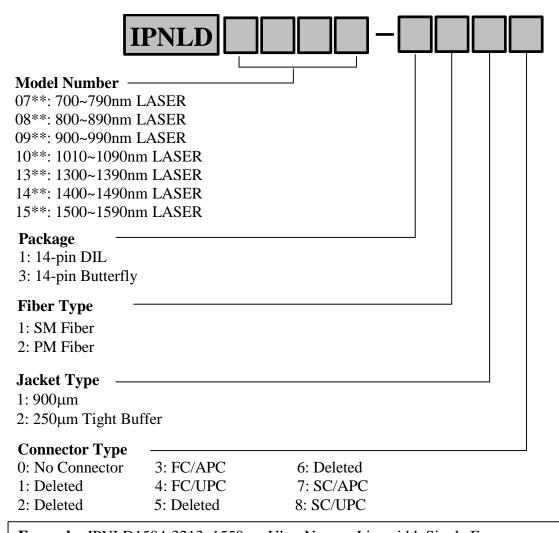
**Example:** IPNLD1504-3213: 1550nm Ultra Narrow Linewidth Single Frequency Laser in 14-pin Butterfly with 900µm PM fiber and FC/APC Connector
